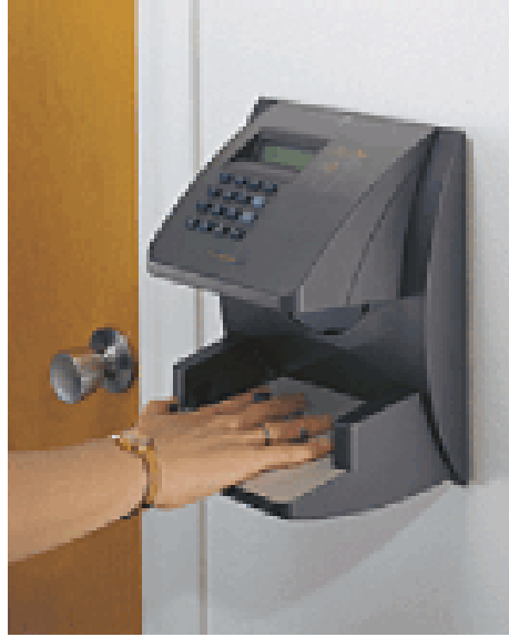
Fig. 7. The HandKey access control device by Recognition Systems Inc.
